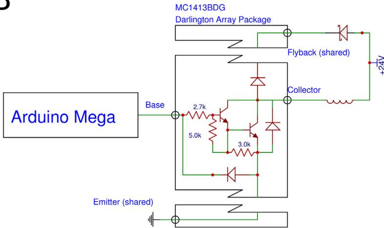
Fig. 4. An electrical schematic of the whole KATARA shield (A) and of a single amplifying circuit on the KATARA shield (B).
