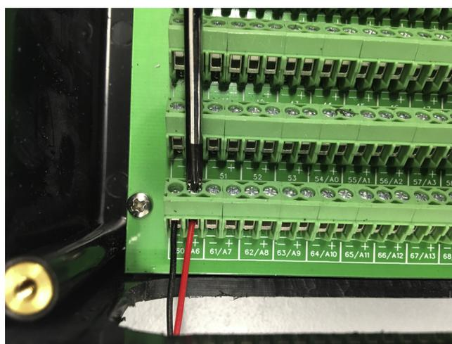
Fig. 8. Solenoid valve lead wires are clamped into place by tightening the screws on the terminal blocks.
