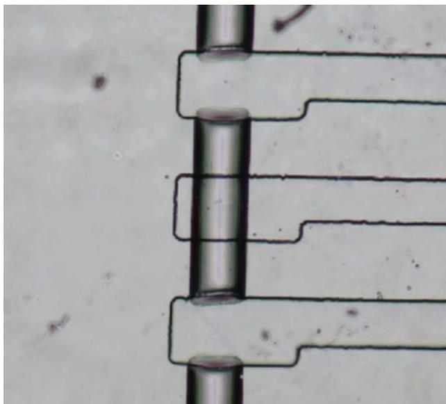
**Video 1.** A peristaltic pump operating at one cycle/second. The frame rate is twenty frames/second. The vertical flow channel is 150 microns wide.
